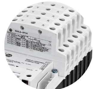
Multiple contactors can be wired together for group operation. Contactors are therefore a good method of controlling blocks of similar loads. Contactors are manufactured to be operated by two types of inputs: a maintained, continuous input requires an electrically held contactor; and a momentary input requiring a mechanically held contactor.
